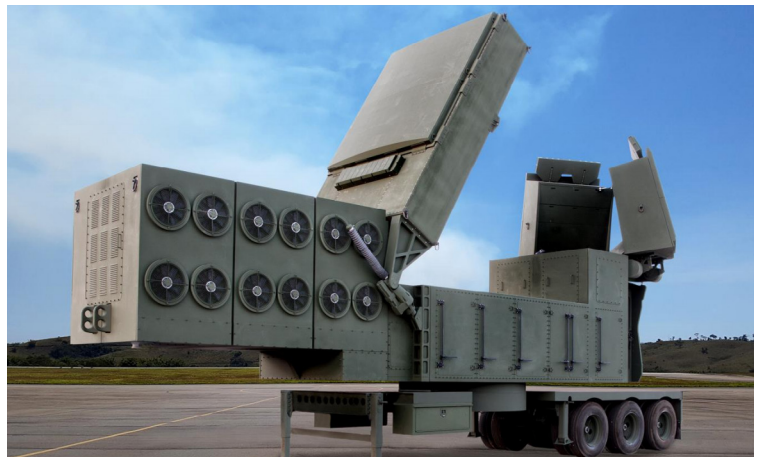
This land-based sensor provides critical information for the long-range classification, discrimination, and identification of missiles.
